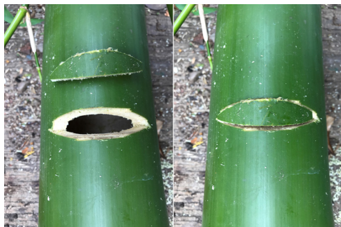
Fig. 4 Openings cut in the culm intersection. Photo: Paulina Maciejewska-Daruk.
